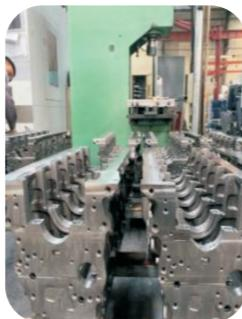
**Side milling -Cylinder block**
