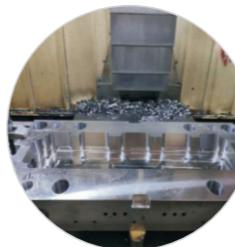
**Side milling -Cylinder block**
