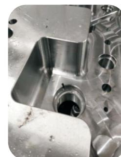
**Application cases****Finish milling - Mould Sidewall**
