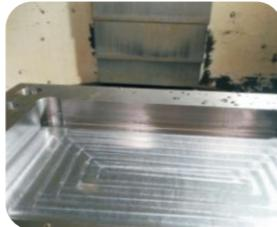
**Roughing - Internal Mould Insert**
